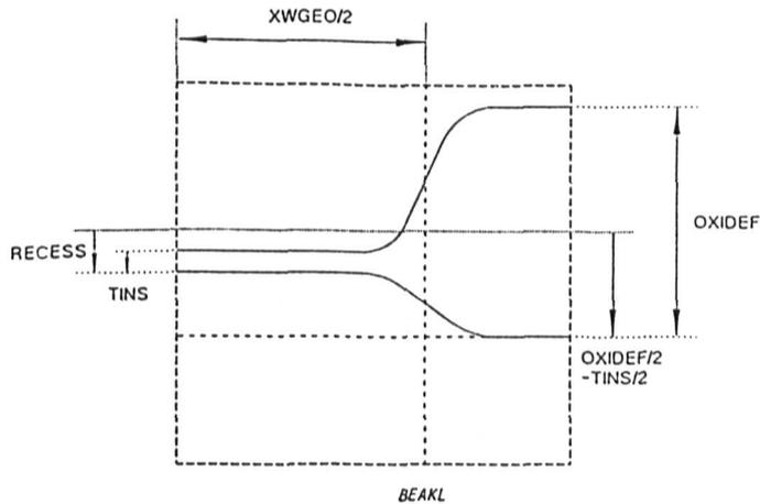
Fig.3 Oxide body parameters in width direction
