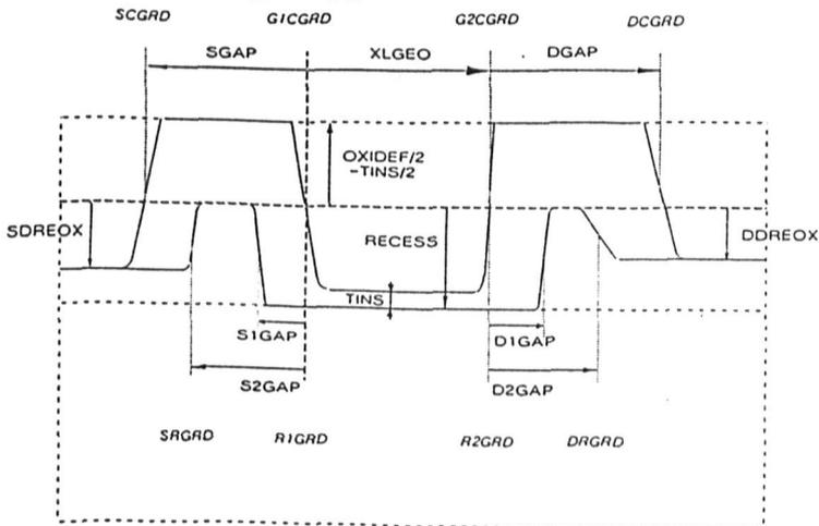
Fig.2 Oxide body parameters in length direction
