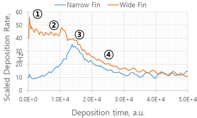
Fig. 7. Effective deposition rate for narrow and wide Fin devices. Key phases of epitaxy are indicated by numbers: 1 – initial stage limited by {111} faceting, 2, 3 – growth rate spikes during structure sidewalls merging for wide and narrow fin devices, respectively; 4 – saturated growth after the formation of a diamond-like shape.
