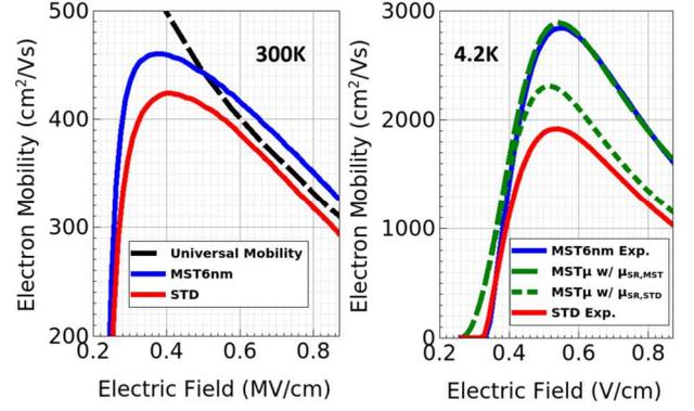
Fig. 4. Mobility analysis. Left: Experimental 300 K mobilities of "STD" and "MST6nm" compared to universal mobility [20]. Right: Experimental 4.2 K mobilities of "STD" and "MST6nm" compared to fitted mobility for MST6nm,  $\mu$ , using either  $\mu_{sr,MST}$  or  $\mu_{sr,STD}$ .
