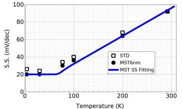
Fig. 5. Subthreshold slope (S.S.) of the "STD" and the "MST6nm" at  $V_D = 50$  mV as a function of temperature. MST fitting curve based on Eq. (5) is also plotted.
