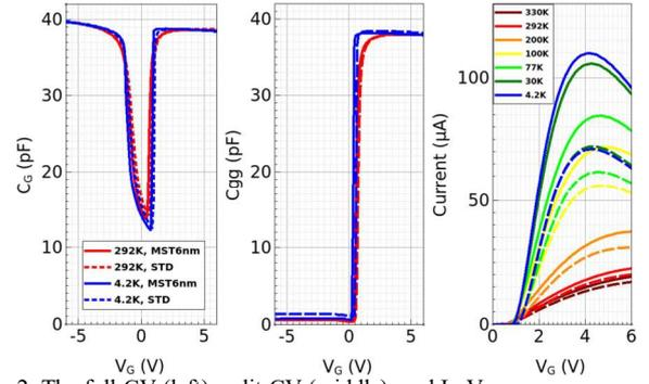
Fig. 2. The full-CV (left), split-CV (middle), and  $I_D$ - $V_G$  curves measured at various temperatures. Dashed lines are "STD" and solid lines are "MST6nm". For clarity, only  $292\ \text{K}$  and  $4.2\ \text{K}$  are shown in the CV curves.  $V_D = 0.05\ \text{mV}$  in the  $I_D$ - $V_G$  measurement.
