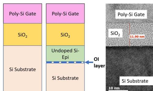
Fig. 1. Illustrations of the gate/channel stack of the baseline "STD" device (left) and the OI "MST" device (middle). The right figure shows a TEM picture of a "MST" device. Note that the OI layers are difficult to see in the TEM because they are partial monolayers and the silicon crystal lattice is maintained.
