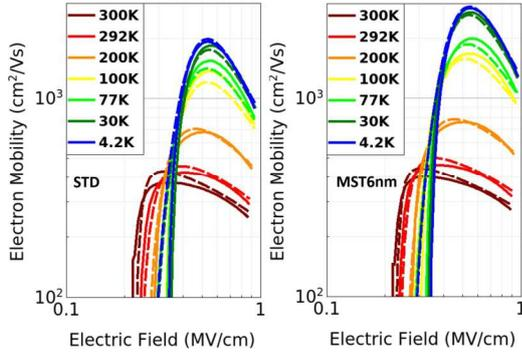
Fig. 3. Electron mobility as a function of temperature and  $E_{\perp}$  for the "STD" (left) and "MST6nm" (right) devices. Solid lines are the mobilities extracted using the  $I_D$ - $V_G$  and split-CV curves. Dashed lines are fitting curves using Eqs. (1)-(4).
