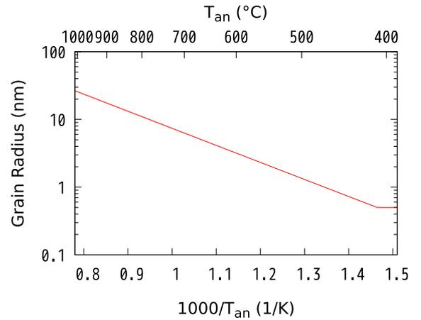
Fig. 2. The grain radius as a function of the annealing temperature. The annealing time is 10 min.
