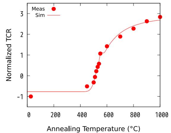
Fig. 6. The TCR of the thin film as a function the annealing temperature. The TCR is normalized by the absolute measured value of the as-deposited sample.
