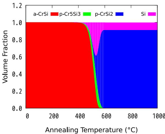
Fig. 4. The volume fraction of each phase. The annealing time is 10 min.
