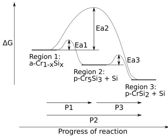
Fig. 1. The schematic diagram of the phase transitions during annealing.
