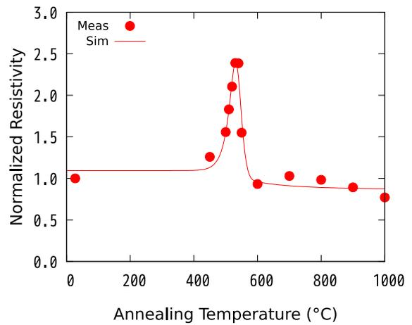
Fig. 5. The resistivity of the thin film as a function the annealing temperature. The resistivity is normalized by the measured value of the as-deposited sample.
