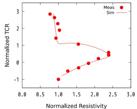
Fig. 7. The dependence of resistivity and TCR on annealing temperature.
