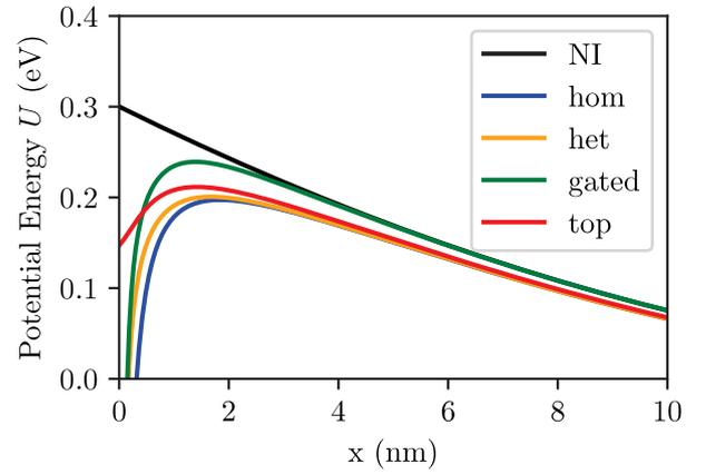
Fig. 5. Potential energy  $U(x) = U_s + U_{\text{image}}$ . The Schottky barrier is plotted in case of no IFBL contributions (NI) and in case of all contact configurations. The surrounding dielectric used for this plot is  $\text{SiO}_2$ .
