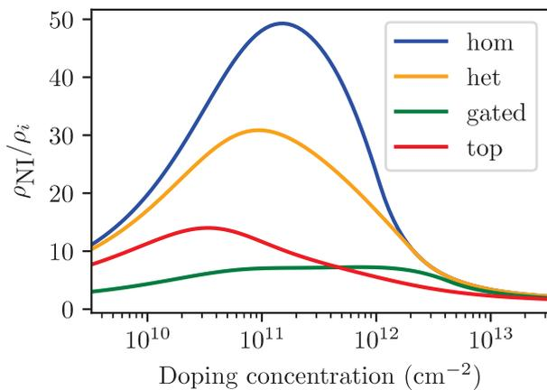
Fig. 8. Ratio of Schottky resistivity w/o IFBL ( $\rho_{NI}$ ) and the resistivity of the various contact configurations ( $\rho_i$ ;  $i =$ ) (a)–(d) for a  $\text{SiO}_2$  surrounding dielectric.
