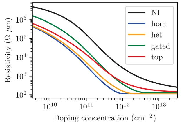
Fig. 6. Contact resistivity vs. doping concentration for a  $\text{SiO}_2$  surrounding dielectric: NI - No IFBL, (a)–(d) with IFBL in all contact configurations.
