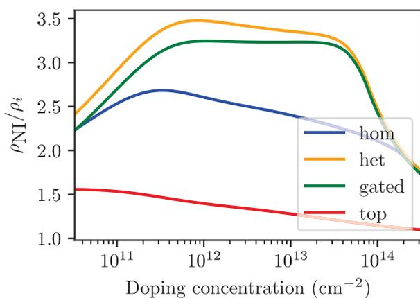
Fig. 9. Ratio of Schottky resistivity w/o IFBL ( $\rho_{NI}$ ) and the resistivity of the various contact configurations ( $\rho_i$ ;  $i =$ ) (a)–(d) for a  $\text{HfO}_2$  surrounding dielectric.
