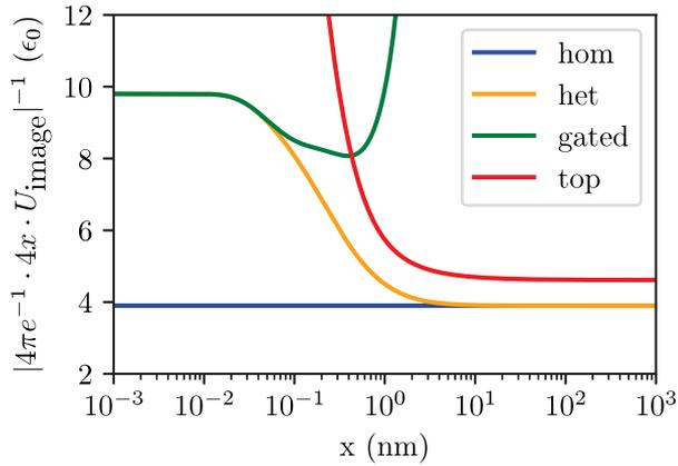
Fig. 4. The “position-dependent” dielectric constant  $\epsilon(x)$  vs.  $x$  for every contact configuration. It compares the behavior of  $U_{\text{image}}$  in each configuration to the expected textbook behavior as defined in Eq. (1).
