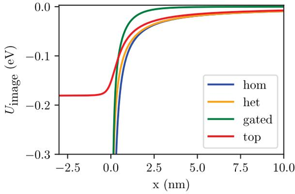
Fig. 3. Image potential energy profiles for the various contact configurations accounting for a surrounding dielectric of  $\text{SiO}_2$ .
