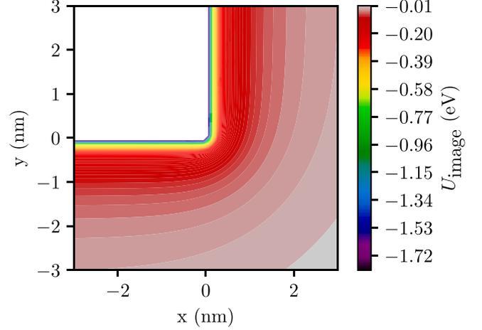
Fig. 2. Image potential energy for a top contact configuration (d), where  $\text{SiO}_2$  is chosen as the surrounding dielectric.
