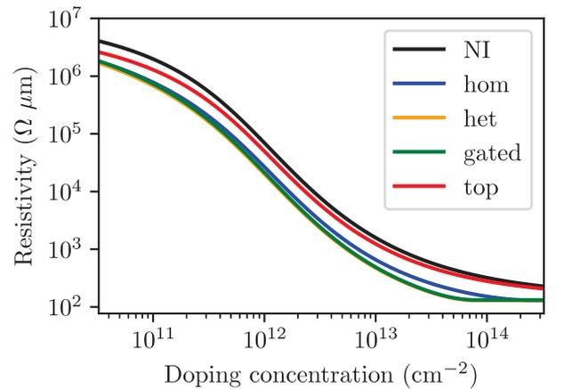
Fig. 7. Contact resistivity vs. doping concentration for a  $\text{HfO}_2$  surrounding dielectric: NI - No IFBL, (a)–(d) with IFBL in all contact configurations.
