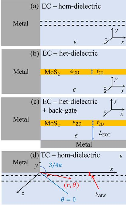
Fig. 1. (a) Edge contact (EC) with homogeneous dielectric (“hom”); (b) EC with heterogeneous dielectric (“het”); (c) EC with heterogeneous dielectric and metal back-gate (“gated”); (d) Top contact (TC) with a homogeneous dielectric (“top”).
