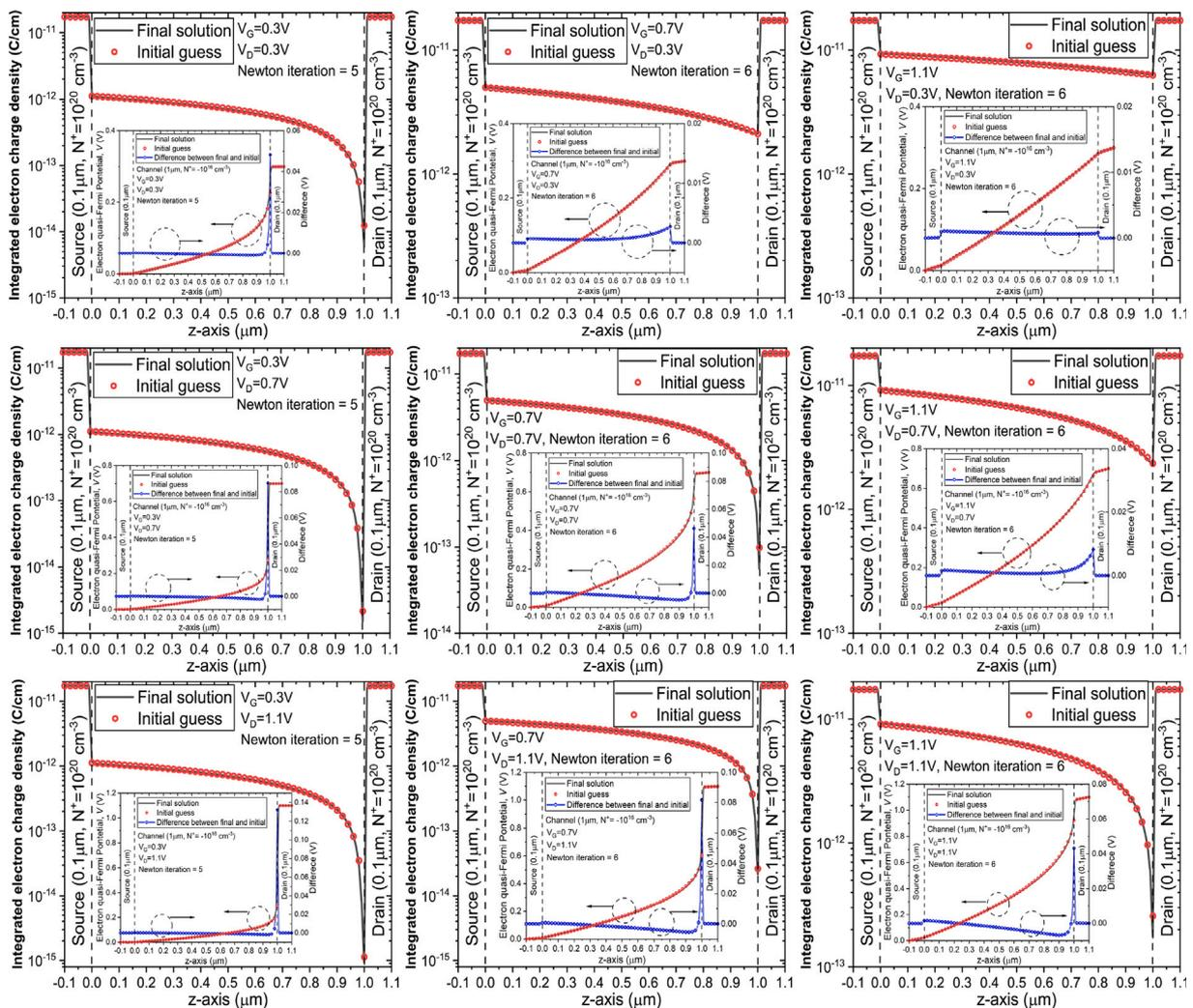
Fig. 4. Initial guesses of  $Q_e$  and  $V$  along the  $z$ -direction compared with final converged results at several bias conditions. The difference of  $V$  between initial guess and final result is also shown. Through the method proposed in this work, at most 6 Newton iterations are needed for solving the drift-diffusion model.
