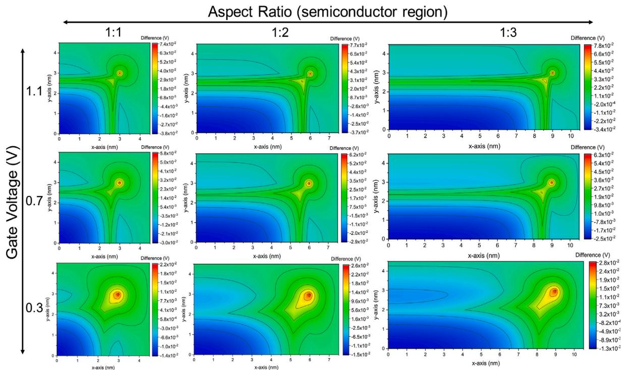
Fig. 2. Difference between the initial guess and the converged solution. Three aspect ratios ( $H:W = 1:1, 1:2,$  and  $1:3$ ) and three gate voltages ( $V_G = 0.3, 0.7,$  and  $1.1 \text{ V}$ ) are considered. Only a quarter of the cross-section is shown. In these examples, the maximum difference is about 77 mV.
