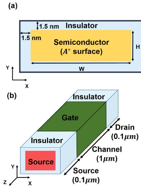
Fig. 1. (a) Cross-section of a rectangular GAA MOSFET and (b) its three-dimensional (3D) structure. The aspect ratio used in this work means a ratio of  $H$  to  $W$ . Thickness of the insulator is 1.5 nm. The channel length is  $1 \mu\text{m}$  and the source/drain region is  $0.1 \mu\text{m}$ -long. The p-type doping concentration of the channel region is  $10^{16} \text{ cm}^{-3}$  and the source/drain n-type doping is  $10^{20} \text{ cm}^{-3}$  in this work.
