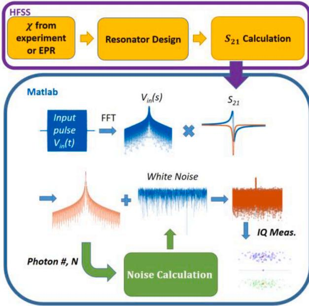
Fig. 2. Illustration of the simulation flow.
