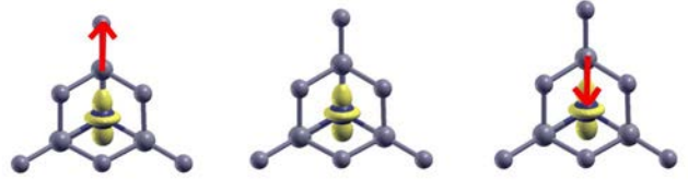
Fig. 2. Jahn-Teller distortions for interstitial Ti in silicon. Red arrows represent the geometry of the elongated (left) and flatted (right) tetrahedron. In yellow, one of the defect t_2 localized electronic states.
