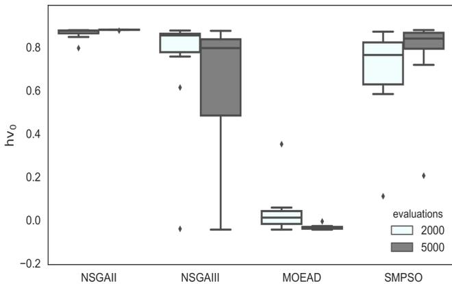
Fig. 3. Comparison of the hypervolume metrics for 10 runs of 2000 and 5000 evaluations using the NSGA-II[14], NSGA-III[15], MOEA/D[17], and SMPSO[18] MOOs.
