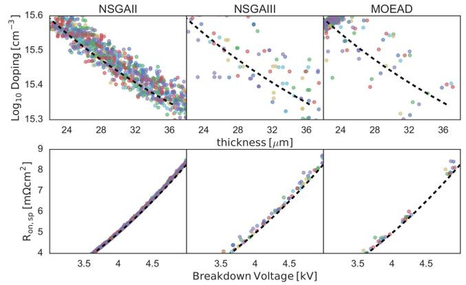
Fig. 4. Comparison of the performance of the MOOs [14],[15],[17] for 10 runs of 5000 evaluations of 0D model. The dashed line represent the approximate design rules from [5]. While [14],[15] obtain a reasonable approximation of the Pareto front, [17] does not fully explore the design space.
