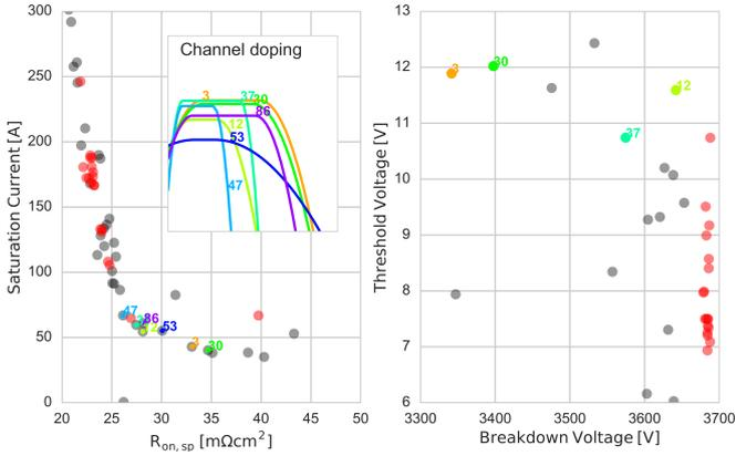
Fig. 6. Trade-off curves between  $r_{on}$  and  $I_{dsat}$  (left) and  $B_V$  and  $V_T$  (right) as the channel of a SiC MOSFET (inset) is varied in a 2D TCAD simulation.
