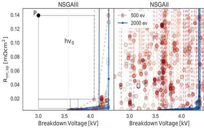
Fig. 2. Comparison of the Pareto fronts found by the NSGA-II[14] (on the right) and NSGA-III[15] (on the left) MOOs for 10 runs of optimization of 0D model for with a limit of 500 evaluations (red dashed lines with circle marker) and 2000 evaluations (blue solid lines with dot marker). Each of the 10 runs is shown with a different shade of color. On the left side, the procedure for the evaluation of the hypervolume for a particular Pareto front is shown.
