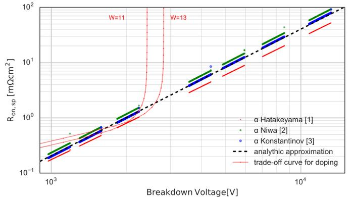
Fig. 1. Trade-off curve between  $r_{on}$  and  $B_V$ . The dots are obtained through MOO optimization[14] of a 0D model with  $\alpha_{n,p}$  from [1][2][3]. The dashed line represents the approximate design rule from [5], obtained through a brute force approach (illustrated by the thin dotted lines).
