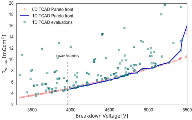
Fig. 5. Trade-off curve between  $r_{on}$  and  $B_V$ . The squares are obtained through MOO optimization[14] of a 1D TCAD model with  $\alpha_{n,p}$  from [3]. The circles indicate the Pareto front shown in Fig. 1 for  $\alpha_{n,p}$  from [3].
