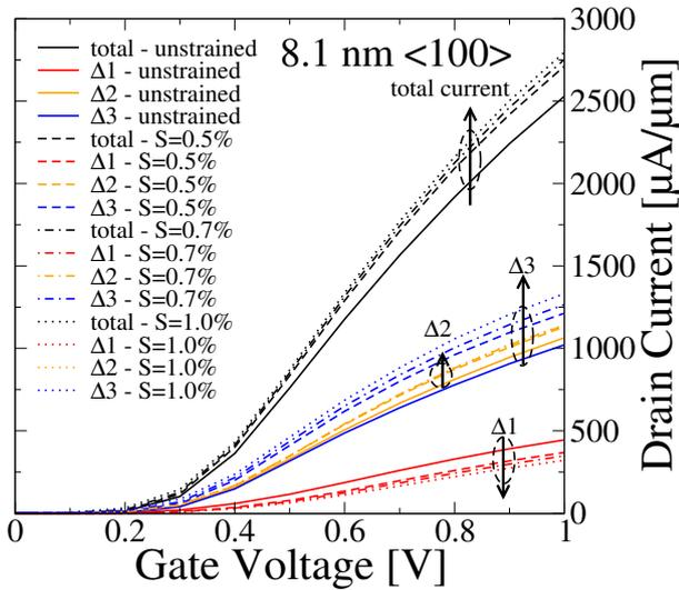
Fig. 5. Valley contributions to the current at  $V_D=0.6$  V in the  $\langle 100 \rangle$  channel orientation under uniaxial  $\langle 100 \rangle$  strain with different strengths (8.1 nm gate device).
