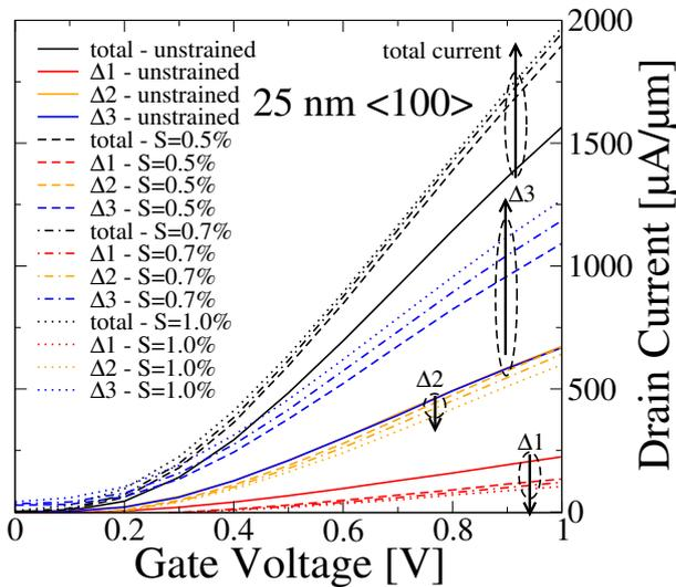
Fig. 6. Valley contributions to the current at  $V_D=1.0$  V in the  $\langle 100 \rangle$  channel orientation under uniaxial  $\langle 100 \rangle$  strain with different strengths (25 nm gate device).
