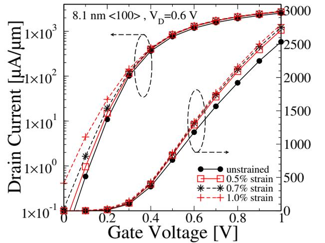
Fig. 4.  $I_D$ - $V_G$  characteristics at  $V_D = 0.6 \text{ V}$  in the  $\langle 100 \rangle$  channel orientation under uniaxial  $\langle 100 \rangle$  strain with different strengths (8.1 nm gate device).
