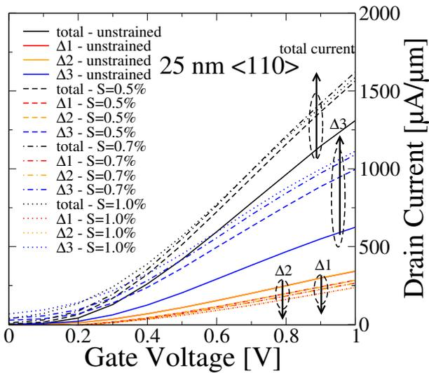
Fig. 9. Valley contributions to the current at  $V_D=1.0$  V in the  $\langle 110 \rangle$  channel orientation under uniaxial  $\langle 110 \rangle$  strain with different strengths (25 nm gate device).
