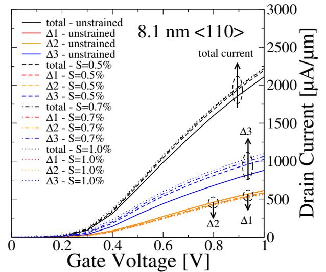
Fig. 8. Valley contributions to the current at  $V_D=0.6$  V in the  $\langle 110 \rangle$  channel orientation under uniaxial  $\langle 110 \rangle$  strain with different strengths (8.1 nm gate device).
