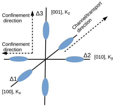
Fig. 3. Six silicon valleys, showing the confinement plane. The transport direction is the  $x$ -axis.
