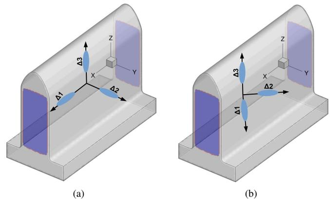
Fig. 2. Conduction band constant energy ellipsoids along  $\Delta$  valleys in silicon for (a)  $\langle 100 \rangle$  and (b)  $\langle 110 \rangle$  channel orientations. Each of the three ellipsoids is double degenerate.
