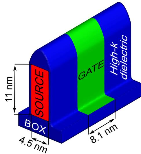
Fig. 1. Schematic of the investigated  $8.1 \text{ nm}$  gate length *n*-channel Si SOI FinFET ( $\text{EOT}=0.55 \text{ nm}$ ).
