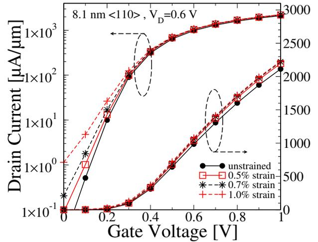
Fig. 7.  $I_D$ - $V_G$  characteristics at  $V_D=0.6$  V in the  $\langle 110 \rangle$  channel orientation under uniaxial  $\langle 110 \rangle$  strain with different strengths (8.1 nm gate device).
