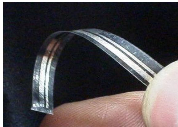
Fig. 1. Photograph of the flexible glucose sensor (width: 3mm) for tear glucose monitoring, which has a sandwich configuration with enzyme membrane, electrolyte membrane, non- and gas permeable membranes, and Pt (narrow metal one) and Ag/AgCl (wide metal one) layers.
