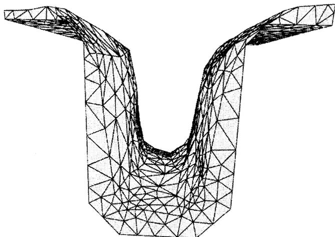
**4:** A surface, extracted from the level set algorithm, already imported in CSG and processed using several logical operations.
