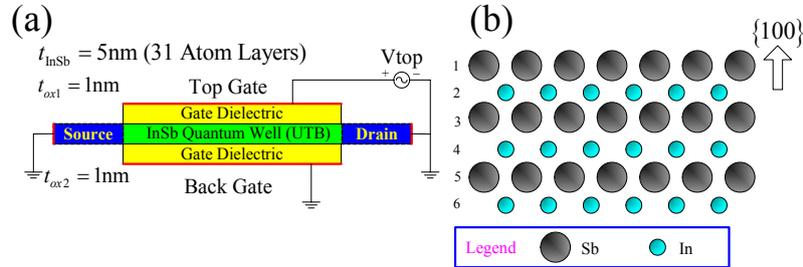
**Figure 1:** (a) The structure of InSb double-gate MOSFET. The channel is undoped and (100) oriented, with a high-k Al<sub>2</sub>O<sub>3</sub> (Aluminum Oxide,  $\epsilon_{ox} = 9.6$ ) gate dielectric. To make our results comparable with other approaches, we adjust the gate-electrode work function such that when both gates are grounded, no potential drop exists and the sheet charge density in the channel is zero. (b) The In and Sb atom layers in the channel.
