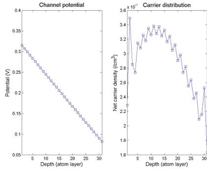
**Figure 3:** Electric potential inside the channel and carrier distribution among all 31 atom layers of InSb channel, calculated by the TB approach with top gate voltage of 0.4V. The serrated charge distribution is induced by the polar chemical bond between In and Sb atom layers.
