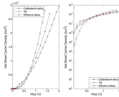
**Figure 4:** Comparison of  $k \cdot p$ , TB, and effective mass (EM) approach in calculating sheet charge density of InSb MOSFET.
