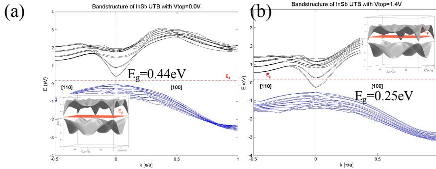
**Figure 2:** Bandstructure calculated using TB method for 5nm InSb channel. The bottom gate is grounded. Top gate voltage is (a) 0V and (b) 1.4V. The insets show the lowest conduction subband and highest valence subband in the Brillouin zone.
