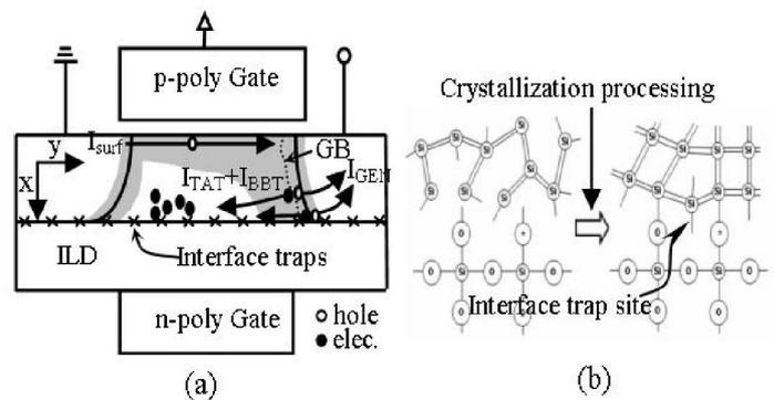
Figure 2. (a) Structure of SC-like SOI pMOSFET on ILD and components of leakage current, (b) Si-O bond structure between SC-like silicon body and ILD before and after crystallization.
