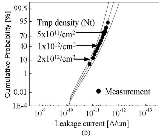
Figure 6. (a) Comparison of the leakage current distribution of SC-like SOI transistor and Bulk-Si transistor. Distribution of SC-like SOI transistor is larger and worse than that of bulk-Si transistor and (b) Effect of trap density ( $N_t$ ) on the leakage current distribution of SC-like SOI transistor. Increase in the trap density reduces the variation of the leakage current distribution, but the magnitude of the leakage current is increased.
