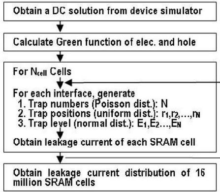
Figure 3. Overall simulation procedure. Trap number obeys the Poisson distribution, their positions are uniformly distributed in the STI-silicon interface and silicon body-ILD interface and their energy levels are normally distributed.
