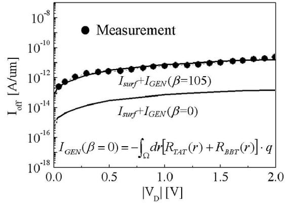
Figure 4.  $V_{Drain}$ - $I_{off}$  curve of the SC-like SOI transistors obtained from the simulation data and measurement. Total leakage current is obtained by generation current ( $I_{GEN}$ ) using the Green's function for  $\beta=0$  and  $\beta=105$ .
