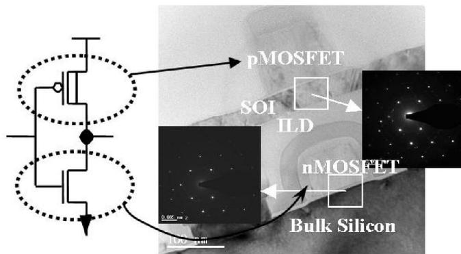
Figure 1. Electron diffraction patterns and TEM image of inverter with stacked SC-like SOI pMOSFET :  $L_{GATE}$  is 80nm and the SC-like Si-body thickness is 25nm.
