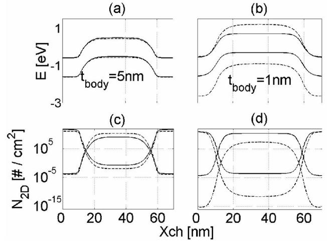
Fig. 3. The conduction & valence bands in the middle ( $t_{\text{body}} / 2$ ) of cell with  $L_{\text{ch}} = 50\text{nm}$  plotted along the channel direction for  $t_{\text{body}} = 5\text{nm}$  (left) &  $t_{\text{body}} = 1\text{nm}$  (right). Dotted and solid lines are result of QB & CL models respectively. The widening of the band gap can be observed with smaller  $t_{\text{body}}$  which decreases the equilibrium carrier concentration.
