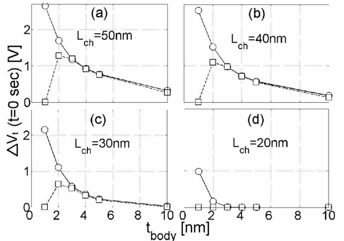
Fig. 4. Change in threshold voltage immediately after **WRITE** ‘0’ for the cells with various dimensions obtained by QB (squares) and CL (circles) models. The models differ significantly at  $t_{\text{body}} < 3\text{nm}$  because of quantum mechanical confinement.
