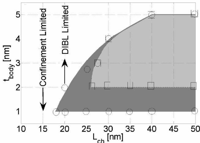
Fig. 5. The allowed design space of 1T-0C cell when dimensions are scaled while keeping  $\Delta V_t \geq 0.3\text{V}$ . The whole area bound by outer curves (circles) is the result of CL model and the lightly shaded area is from QB model (squares). The dark shaded area is where the two models differ due to the effect of charge confinement. At higher  $t_{body}$ , DIBL limits the design space while at  $t_{body} \leq 2\text{nm}$ , quantum confinement limits the design.
