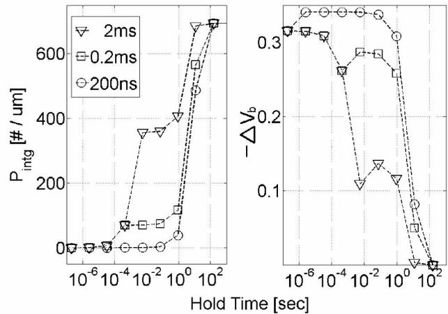
Fig. 6. The effect of WRITE '1' drain disturb on 1T-0C cell in HOLD '0' with  $L_{ch} = 50\text{nm}$  and  $t_{body} = 10\text{nm}$ .  $P_{intg}$  (left) and  $-\Delta V_b$  (right) are plotted as a function of hold time for cumulative disturb times of 200ns, 0.2ms and 2ms with higher values reducing sense margin and retention time.
