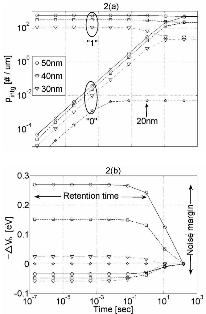
Fig. 2.  $P_{intg}$  (2a) and  $\Delta V_b$  (2b) in **HOLD** state after **WRITE** '0' plotted as a function of **HOLD** time in 1T-0C cell of  $t_{body} = 10nm$  with various  $L_{ch}$ . The effect of DIBL is prominent in smaller  $L_{ch}$  where the  $\Delta V_b$  gap becomes smaller and results in decreased sense margins.
