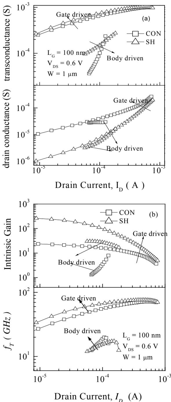
Figure 7(a) Device transconductance and drain output conductance, (b) Intrinsic gain and cut-off frequency ( $f_T$ ) as a function of bias current for gate and bulk driven device with CON and SH doping. Transistor width is taken as 1  $\mu$ m and drain bias is kept at 0.6 V.
