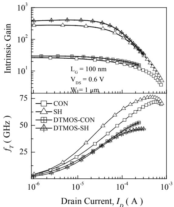
Figure 4. Device intrinsic gain and  $f_T$  as a function of bias current for all the devices with CON and SH doping. All the devices are simulated in PDSOI mode.
