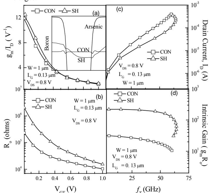
Figure 1. (a) Device  $g_m/I_D$  and (b) output resistance ( $R_o$ ) as a function of gate overdrive ( $V_{GT}$ ), (c) drain current requirement and (d) Intrinsic gain as a function of device cut-off frequency for both CON and SH devices.
