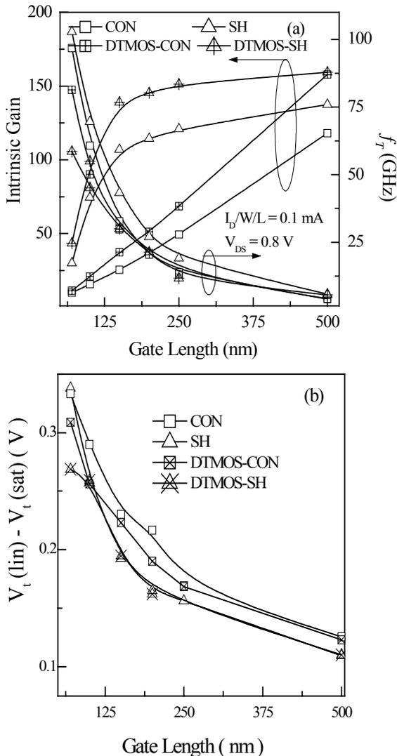
Figure 5(a) Device intrinsic gain and cut-off frequency as a function of gate length at  $I_D/W/L = 0.1 \text{ mA}$ , (b) DIBL as of gate length for all the devices. DIBL is quantified as the change in the  $V_t$  for a change of 1V in drain voltage.
