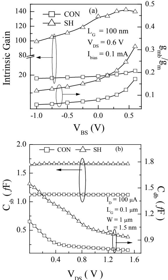
Figure 2(a) Device intrinsic gain and  $g_{mb}/g_m$  as a function of body bias, (b) source-to-body ( $C_{sb}$ ) and drain-to-body capacitance ( $C_{db}$ ) as a function of drain voltage for both CON and SH devices.
