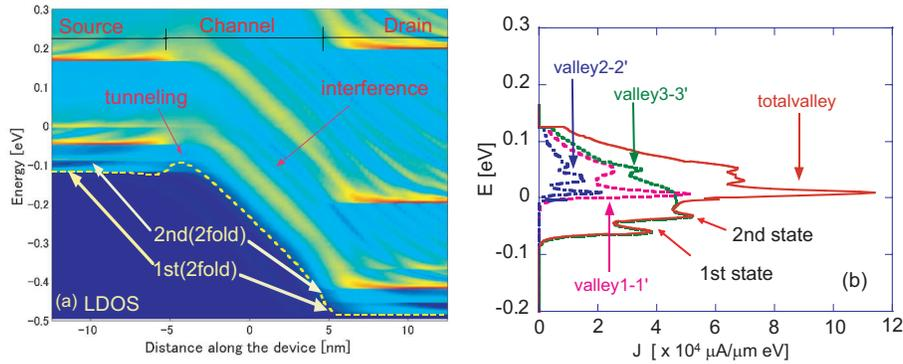
Figure 3: (a) Local density of states in the device under  $V_{gt} = V_{gb} = 1.0$  V and  $V_{ds} = 0.4$  V. “2 fold” stands for valleys 3-3’ which have heavy effective mass in the confinement direction whereas light effective in the transport direction. (b) Energy spectrum of the current density. The 1st and 2nd subbands indicated by arrows are those of the 2 fold valleys.
