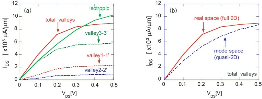
Figure 2: (a)  $I$ - $V$  characteristics taking account of the anisotropic effective masses (total valleys) compared to those with an isotropic effective mass (isotropic). (b) Comparison of  $I$ - $V$  characteristics of the real-space solution (solid line) with the mode-space solution (dashed line). ( $V_{gt} = V_{gb} = 1.0$  V).
