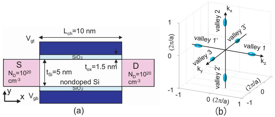
Figure 1: (a) Schematic structure of a DG MOSFET under investigation.  $L_{\text{gtop}} = L_{\text{gbot}} = 10 \text{ nm}$ ,  $t_{\text{Si}} = 5 \text{ nm}$ ,  $t_{\text{ox}} = 1.5 \text{ nm}$ ,  $N_{\text{D}} = 1.0 \times 10^{20} \text{ cm}^{-3}$  are assumed. (b) 6 rotated ellipsoids in Si band structure.
