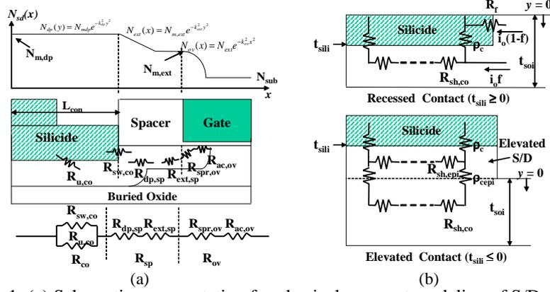
Figure 1: (a) Schematic representation for physical compact modeling of S/D extrinsic resistance and (b) recessed and elevated silicide contact cross-section with modified tri-layer TLM network model.
