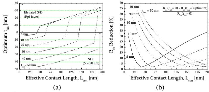
Figure 5: (a) Guideline for optimum silicide contact location as a function of effective contact length in elevated S/D contact structure and (b) resistance improvement at optimum  $t_{sili}$  with respect to  $t_{sili} = 0$  nm.
