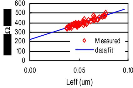
Figure 2: Measured S/D extrinsic resistance data of NMOSFET for model calibration and TCAD simulation.
