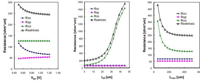
Figure 3: Modeling analysis of S/D extrinsic resistance and components calibrated with measured and simulation data. Significant  $R_{co}$  contribution ( $> 50\%$ ) is observed.
