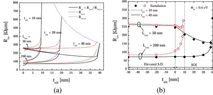
Figure 4: (a) Contact resistance behavior according to effective contact length and (b) its simulation verification for elevated contact with  $t_{soi} = 10$  and  $40$  nm.
