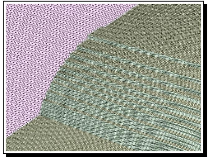
Fig. 2. Process front after marching cube discretization (332718 triangles)
