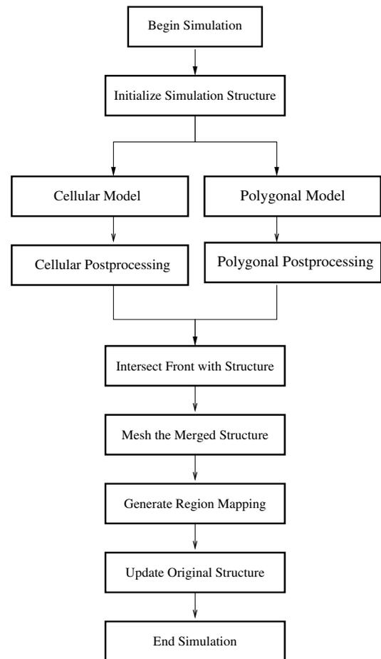
Fig. 1. Simulation flow of **TOPO3D**
