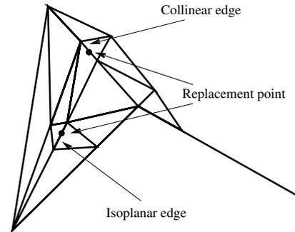
Fig. 6. Illustration of the edge removal algorithm in the coarsening stage
