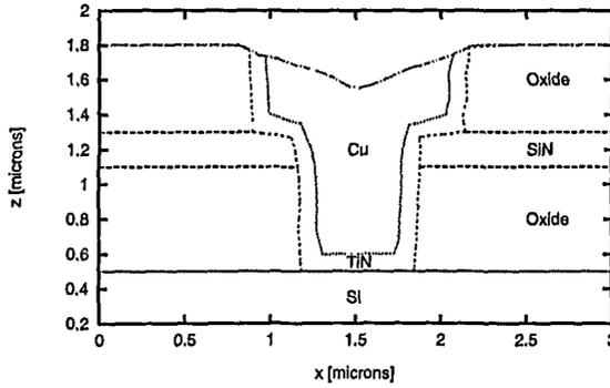
Figure 3: Cross section through the middle of one of the contact holes.
