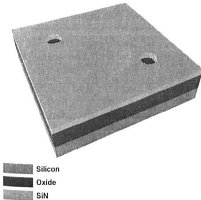
Figure 1: Geometry after patterning the SiN layer at the contact hole positions.
