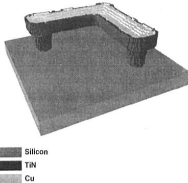
Figure 2: Geometry of the contacts with interconnecting lines. The oxide and nitride layers are not shown.
