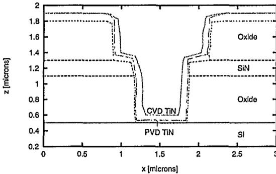
Figure 4: Barrier deposited by CVD in comparison with barrier deposited by collimated sputtering (PVD).
