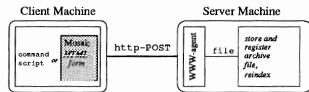
Figure 2: Uploading data to the server is performed by http-POST to WWW-agents (CGI-scripts).
