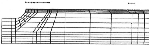
FIGURE 5: Hybrid Mesh for On-Resistance Calculations
