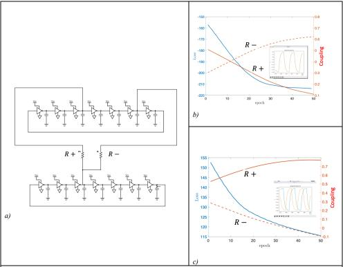
Fig 1. Machine learning the phase relations in a two-oscillator system. In order to couple the two Ros in phase, their like nodes should strongly couple, meaning that the R+ resistance should be small and R- large. For anti-phase coupling, R- should couple strongly, while R+ should be large. The machine learning algorithm adjusts the resistances until this state is reached, as shown in b) and c).
