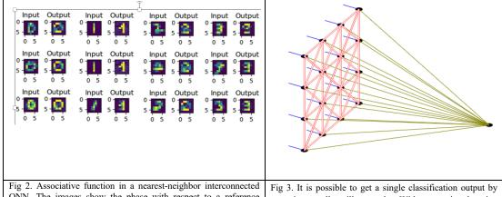
ONN. The images show the phase with respect to a reference oscillator. In most (but not all) cases the distorted digits (handwritten images) converge to the target digits.
