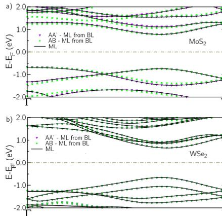
Fig.5: Comparison between monolayer bands (solid line) and extracted bands from the heterostructure bilayer Hamiltonian for a) MoS<sub>2</sub> and b) WSe<sub>2</sub> for the different stacking considered.
