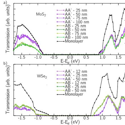
Fig.4: Transmission coefficient for a) MoS<sub>2</sub> and b) WSe<sub>2</sub> for the two different stacking considered and for overlapping length ranging from 12 nm till 100 nm. For comparison the monolayer transmission is reported for both materials.
