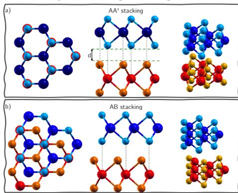
Fig.2: Different TMDs stacking considered a) AA' and b) AB.
