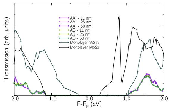
Fig.6: Transmission coefficient for the MoS<sub>2</sub>-WSe<sub>2</sub> heterostructure for different overlapping lengths for the two stackings considered. Monolayer of isolated MoS<sub>2</sub> and WSe<sub>2</sub> are reported for reference.
