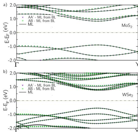
Fig.3: Comparison between monolayer bands (solid line) and extracted bands from bilayer Hamiltonian for a) MoS<sub>2</sub> and b) WSe<sub>2</sub> for the different stacking considered.
