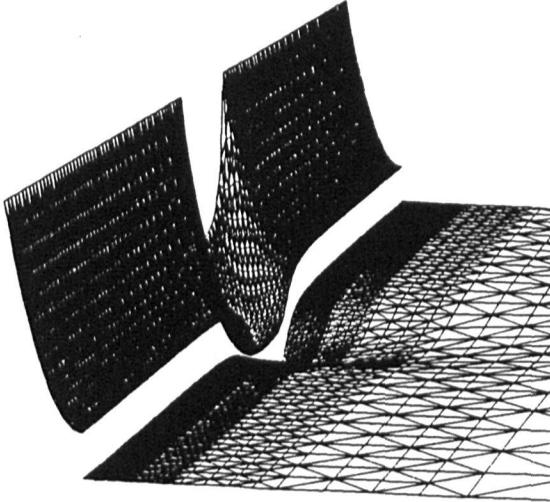
Figure 3: Sample result of the potential landscape in the semiconductor region. Shown is the conduction band obtained by the FBEM algorithm for  $-1.0V$  gate bias. The heterointerface is clearly visible at the discontinuity of the potential.
