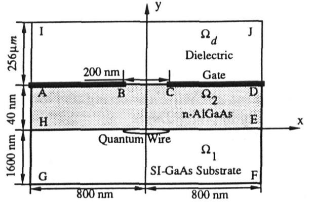
Figure 2: The problem domain consisting of the semiconductor regions,  $\Omega_1$  and  $\Omega_2$ , and the dielectric region,  $\Omega_d$ . the semiconductor exposed surface B-C is treated as the interface between the semiconductor and the dielectric.
