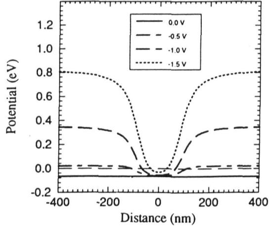
Figure 4: Result of the FBEM algorithm showing the conduction band profiles parallel to the heterointerface (on the GaAs side) for different bias conditions.
