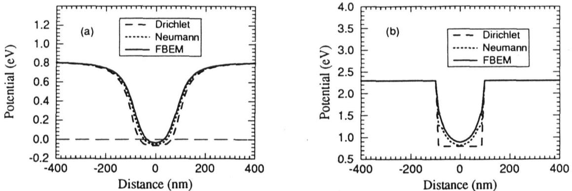
Figure 5: Comparison of the conduction band profiles under  $-1.5$  V gate bias for the three types of boundary conditions on the exposed semiconductor surface; (a) parallel to the heterointerface (on the GaAs side), and (b) parallel to the semiconductor surface.
