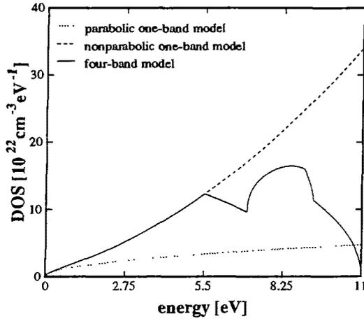
Figure 1. DOS of different band-structures used for SiO<sub>2</sub>.
