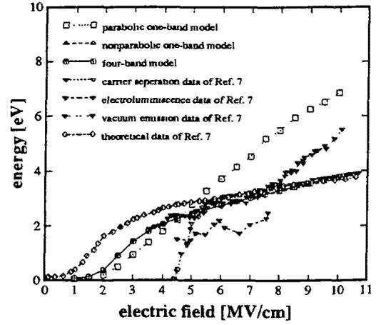
Figure 4. Mean kinetic energy in SiO<sub>2</sub> compared with the data of Ref. 7.
