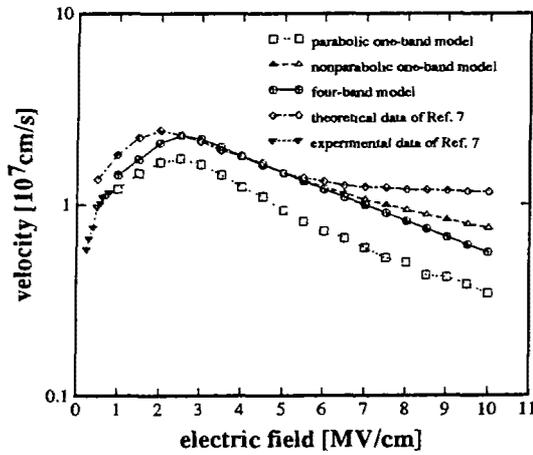
Figure 3. Drift velocity of different band-structures in SiO<sub>2</sub>.
