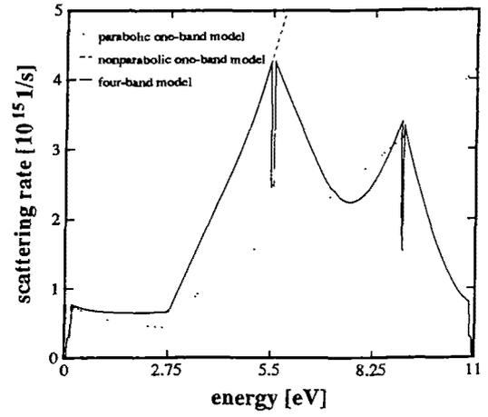
Figure 2. Scattering rates of different band-structures used for SiO<sub>2</sub>
