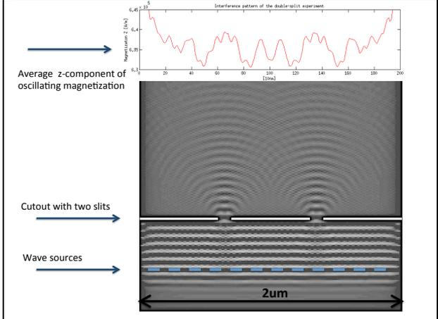
Fig. 4. A double-slit interference pattern from spin waves
