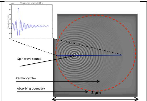
Fig. 2. Spin-wave distribution generated by a single 30 nm diameter spin-torque source. The source is placed on a 5 nm thick Permalloy film. There is a constant 1.0 T magnetic film pointing  $80^\circ$  to the film plane. The decay of spin wave intensity is close to a  $1/r$  law, as expected from a point source.
