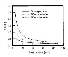
Figure 4: The calculated parasitic capacitance for the three interconnects with different line space.
