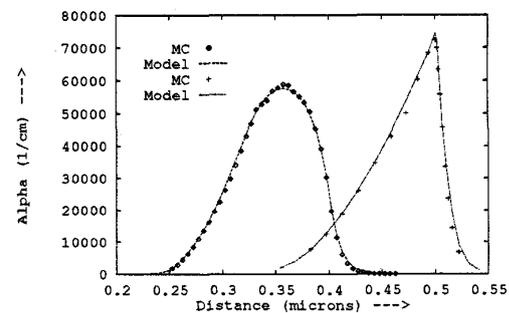
Figure 4: Comparison between II coefficients obtained from MC and our model for an abrupt profile and an LDD profile.
