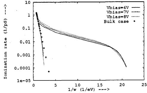
Figure 2: Impact Ionization rates obtained from self-consistent MC simulations of an abrupt  $n^+ - n^- - n^+$  device vs. total average electron energy.
