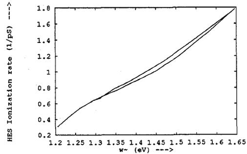
Figure 3: II rate vs. average energy of the high energy electron subpopulation (case of widest hysteresis loop).
