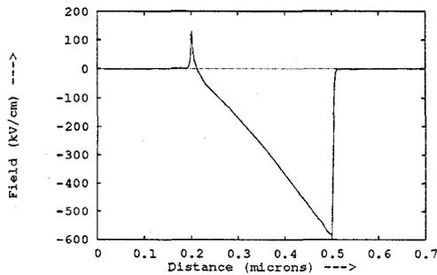
Figure 1: Field profile for self-consistent MC simulations of an abrupt  $n^+ - n^- - n^+$  device at  $V_{bias} = 8V$ .
