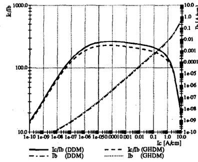
Figure 2: Gain  $I_C/I_B$  and  $I_B$  at  $V_{CB} = 1V$
