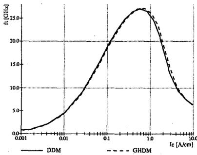
Figure 3: Common base  $f_T$  at  $V_{CB} = 1V$
