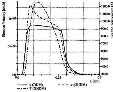
Figure 1: Electron temperature and velocity within intrinsic transistor at  $V_{BE} = 0.8V$ ,  $V_{CE} = 1.4V$
