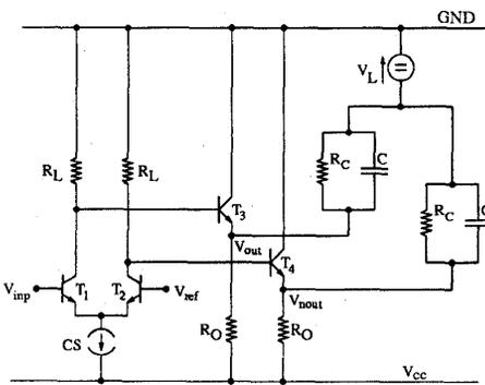
Figure 5: ECL-inverter circuit:  $V_{CC} = -3.3V$ ,  $V_{ref} = -1.087V$ ,  $V_L = -1.087V$ ,  $C_S = 0.6mA$ ,  $R_L = 0.672K\Omega$ ,  $R_O = 4.036K\Omega$ ,  $R_C = 95.7K\Omega$ ,  $C = 14.2fF$
