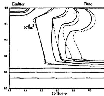
Figure 4: Plot of electron density equiconcentration lines for  $V_{CB} = 1V$ ,  $I_C = 0.73A/cm$  and the different device models (neighboring lines differ by a factor of 10; drawn line: DDM; dashed dotted: GHDM)
