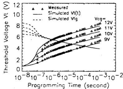
Figure 3: Calculated and measured programming characteristics  $V_i(t)$  for a  $0.5\mu m$  EPROM device. It took only 1 second CUP time on Sun SPARC2 to calculate these four curves using the PPQT method.
