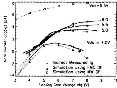
Figure 5: Calculated and measured gate current  $I_g$  for  $0.5\mu m$  EPROM device. Excellent agreement to the measured data has been obtained by using a fitted Monte Carlo (FMC) electron energy distribution function, while the results using original Maxwellian (WM) distribution are more than three orders of magnitude higher than the measured data.
