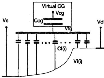
Figure 1: The discretized gate capacitor EPROM model, where the  $C_{fg}(i)$  is defined by numerical mesh of device simulation, and the "virtual control gate" is not physically simulated by numerical device simulation.
