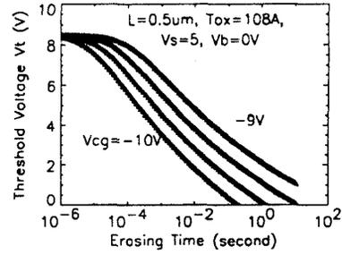
Figure 4: Calculated erasing characteristics for a  $0.5\mu m$  Flash EPROM device.
