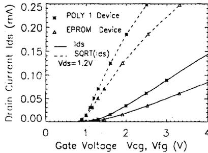
Figure 2: Calculated threshold characteristics for both Poly-1 and EPROM devices with  $L=0.5\mu m$ .
