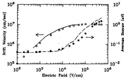
Fig. 5. Electron drift velocity and average energy in bulk silicon computed with the present model (circles); solid line : experimental drift velocity[12], broken line : MC calculated average energy[2].
