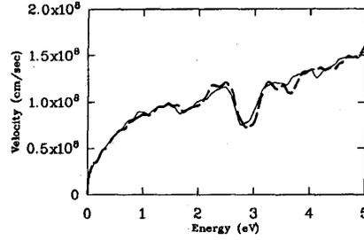
Fig. 2. Electron  $U_g(E)$  calculated using EPM (solid line);  $U_g(E)$  of present model (broken line).
