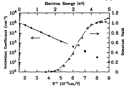
Fig. 6. Impact ionization coefficients and quantum yield; lines : experiments, circles: simulations. Solid line and solid circles : impact ionization[7], broken line and open circles : quantum yield [8]
