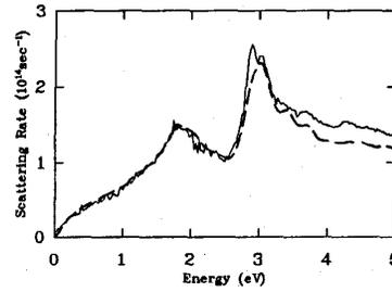
Fig. 4. Total phonon scattering rate : broken line : present model; solid line : Fischetti et al.[2].
