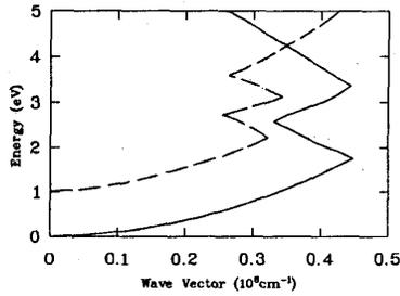
Fig. 3. Generated isotropic E-k relations for X band (solid line) and L band (broken line).
