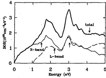
Fig. 1. Total DOS( $E$ ) calculated using EPM (thick solid line) is same with the sum of  $D_X(E)$  and  $D_L(E)$ ; solid line :  $D_X(E)$ , broken line :  $D_L(E)$ .
