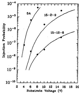
Fig. 7. Injection probability vs. substrate voltage for  $E_{ox} = 2MV/cm$  and three different devices. Lines : experiments [8], circles : simulations.
