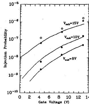
Fig. 8. Injection probability vs. gate voltage for three different substrate voltages. Lines : experiments [9], circles : simulations.
