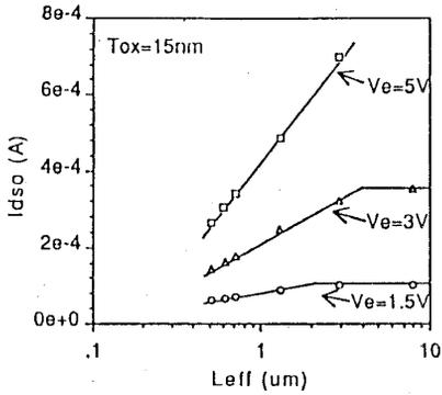
Fig1. Experimental  $I_{dso}$ - $L_{eff}$  relationship measured MOSFETs fabricated by a 0.5um process
