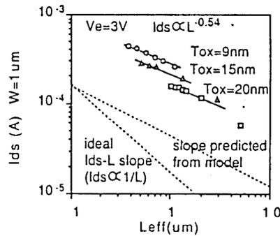
Fig7. Comparison between experiments and proposed model on  $I_{ds}(W=\text{const.})$ - $L$  curves
