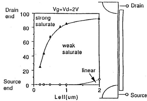
Fig5. Classified lateral field effects on the carrier (electron) flow along the channel region
