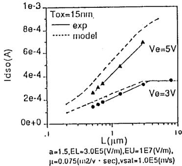
Fig6. Experimental verifications of  $I_{dso}$  degradation in short channel structure
