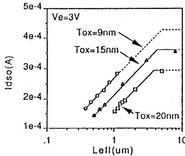
Fig2. Experimental  $I_{dso}$ - $L_{eff}$  relationship obtained with devices fabricated by 0.2-1.3um process levels
