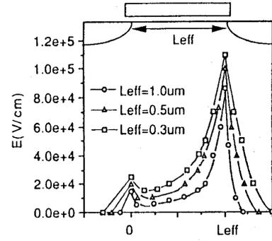
Fig3. Lateral field distribution analysis for  $L_{eff}=0.3, 0.5, 1.0$ um MOSFETs
