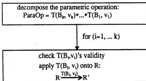
Figure 4 - Parametric Operation Algorithm
