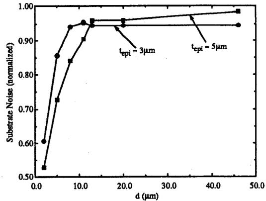
Figure 2 - Substrate Noise vs. Epitaxy Thickness and Guard Ring Distance
