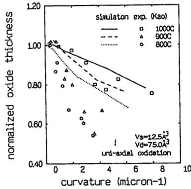
Fig.4 Normalized oxide thickness as a function of curvature.
