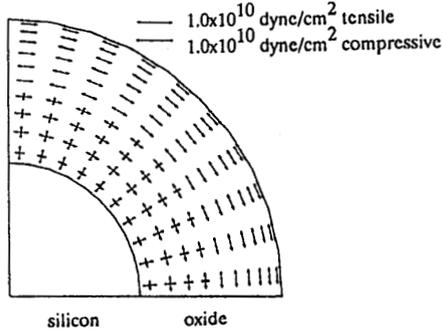
Fig.3 Principal stress in the oxide formed on a cylindrical substrate.
