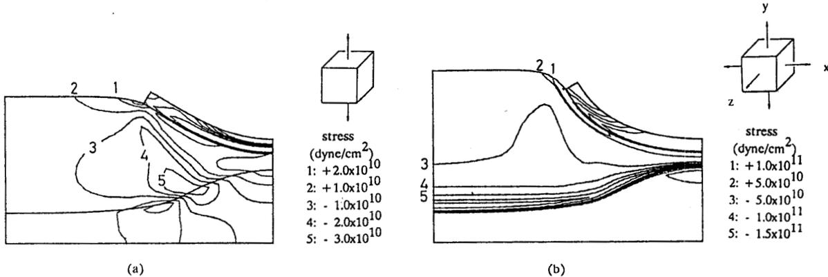
Fig.5 x-component of the stress in LOCOS structure (950C wet). (a) uniaxial oxidation; (b) dilational oxidation.
