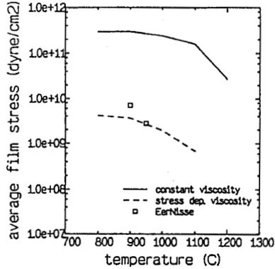
Fig.2 Average film stress as a function of oxidation temperature.
