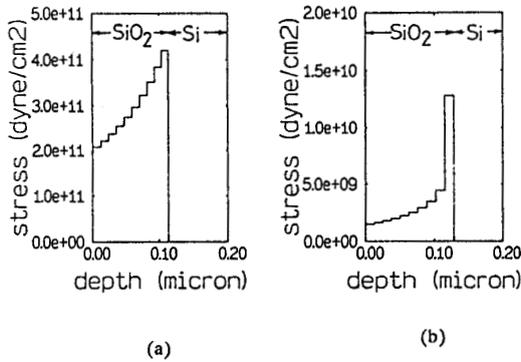
Fig.1. Plots of the stresses induced by planar oxidation. (a) constant viscosity; (b) shear-stress-dependent viscosity.
