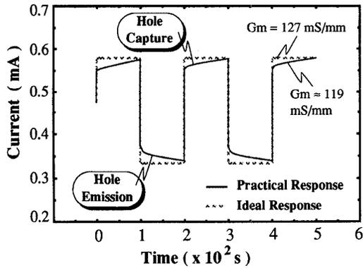
Fig. 3 (a) Pulse Narrowing due to Hole-Trap on the Surface
