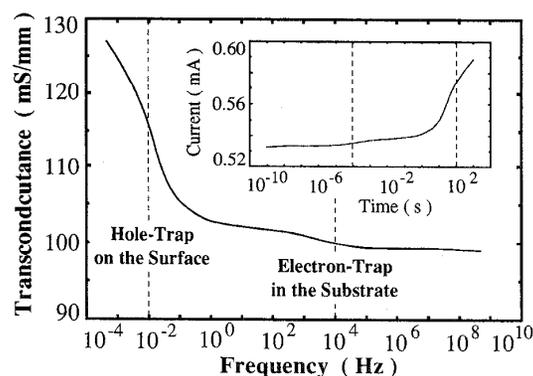
Fig. 2 Frequency Dispersion of Transconductance and Transient Current in Response to a Step Bias
