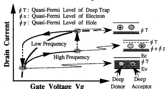
Fig. 1 (a) Hysteresis of Current-Voltage Characteristics in Gate Lag
