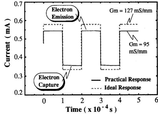
Fig. 3 (b) Pulse Narrowing due to Electron-Trap in the Substrate
