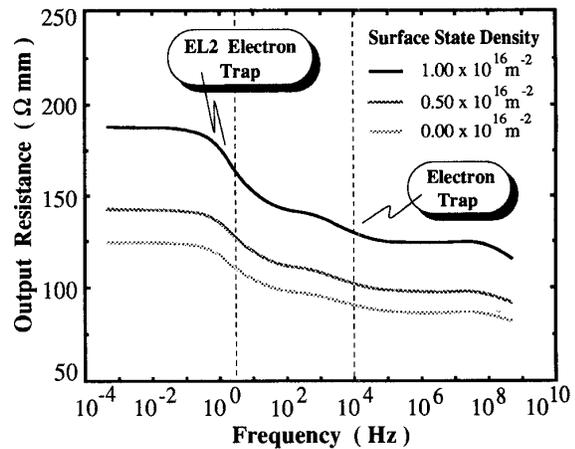
Fig. 4 Multiple Frequency Dispersions of Output Resistance
