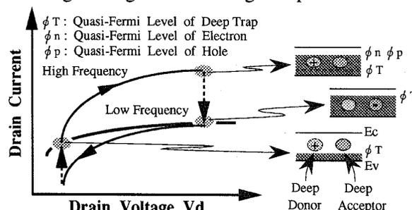
Fig. 1 (b) Hysteresis of Current-Voltage Characteristics in Drain Lag
