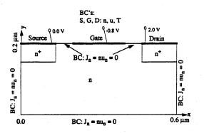
Fig 1. A two dimensional MESFET example
