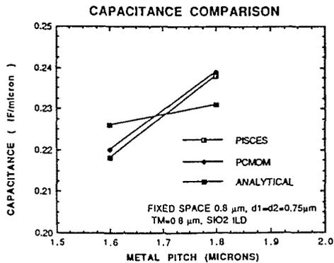
FIG 3. CAPACITANCE COMPARISON OF PISCES PCMOM AND ANALYTICAL METHODS
