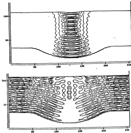
Figure 6. PAC contours for positive and negative polarity resist for a contact hole on a curved substrate.
