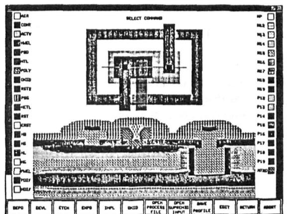
Figure 9. Bipolar Transistor with collector plug "stitch-back"
