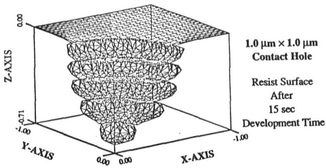
Figure 4. 3-D development of a contact hole.
