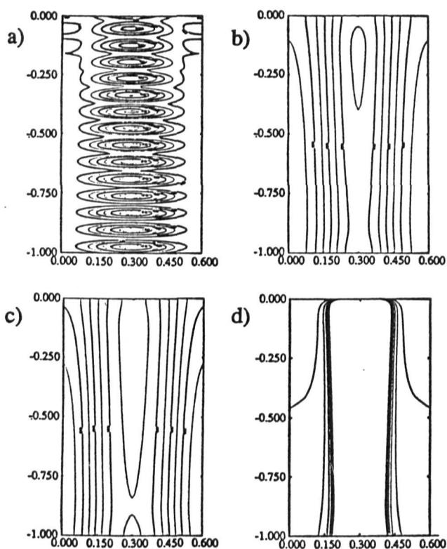
Figure 2. Simulation of 0.3 um line/space profiles in 1.0 um SNR-248N a) exposure, b) diffusion of photo-generated acid, c) cross-linking, and d) development.
