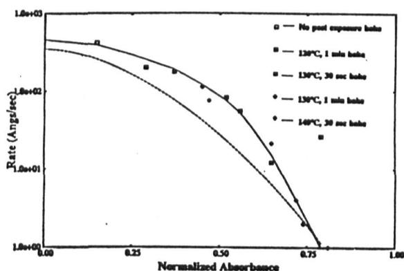
Figure 1. Dissolution rate versus IR absorbance for electron-beam and optical exposure.
