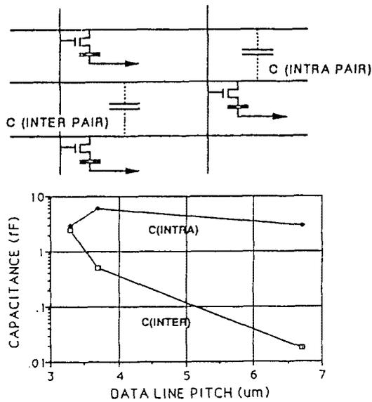
Fig. 1 Three-dimensional simulation of data-line capacitances in DRAM.
