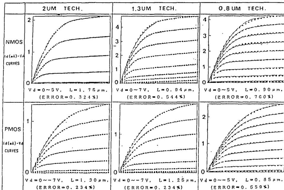
Fig. 3 Comparison of I-V curves between experiments and the MOSTSM model.
