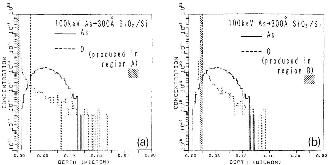
Figure 2. Simulation results for 100keV As implantation into silicon through a 300Å-thick SiO<sub>2</sub> layer. The oxide layer was divided into five 60Å-thick sub-layers. (a) Oxygen distribution (broken line), recoiling from top 60Å surface sub-layer (region A). (b) Oxygen distribution (broken line), recoiling from the inside 60Å-thick sub-layer (region B).
