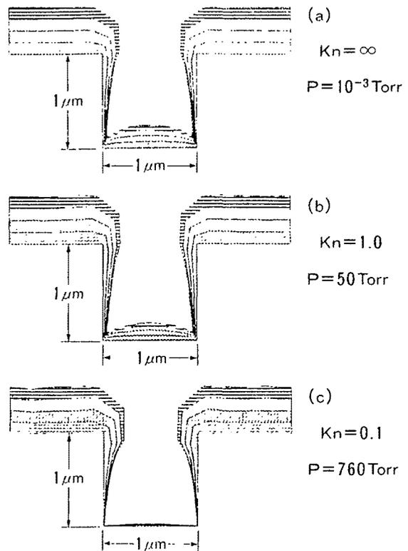
Fig.2 Simulated time evolution of surface contours for CVD -- the effect of the Knudsen number  $Kn$  ( $P_{sr} = 1.0$ )<sup>11)</sup>
