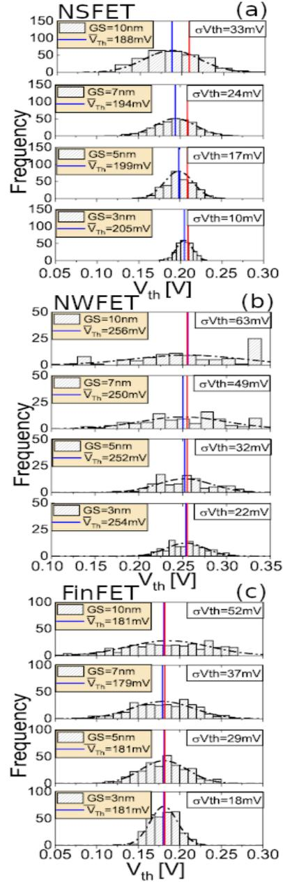
Figure 2. Threshold voltage ( $V_{Th}$ ) histograms due to the MGG for different grain sizes (GS) for (a) the 12 nm gate length NSFET, (b) the 10 nm gate length NWFET, and (c) the 10.7 nm gate length FinFET.  $\sigma V_{Th}$  is the threshold voltage standard deviation,  $\bar{V}_{Th}$  the mean values of the distributions (blue line), and  $V_{Th,ideal}$  the idealistic value of the device with a uniform gate (WF=4.52 eV): 209 mV for NSFET, 255 mV for NWFET, and 182 mV for FinFET.
