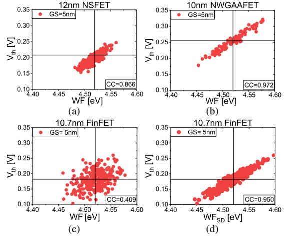
Figure 4. Scatter plot between the  $V_{Th}$  and the mean WF of the gate for each MGG profile at a GS=5 nm for (a) the 12 nm NSFET, (b) the 10 nm NWFET, (c) the 10.7 nm FinFET, and (d) the 10.7 nm FinFET with the mean WF of SD grains ( $WF_{SD}$ ). The black lines represent the continuous WF of 4.52 eV and his associated  $V_{Th,ideal}$ .  $CC$  is the Pearson's correlation coefficient.
