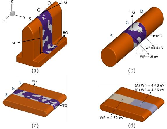
Figure 1. 3D schemes of the different architectures affected by arbitrary MGG (metal grain granularity) profiles. Realistic metal gate configurations are shown for (a) the 10.7 nm gate length FinFET, showing the sidewalls of the gate (SD), the top of the gate (TG), and the bottom of the gate (BG), (b) the 10 nm gate length NWFET, and (c) the 12 nm gate length NSFET. (d) A scheme of the 12 nm gate length NSFET affected with a synthetic MGG profile, showing the two hypothetical cases (A), and (B).
