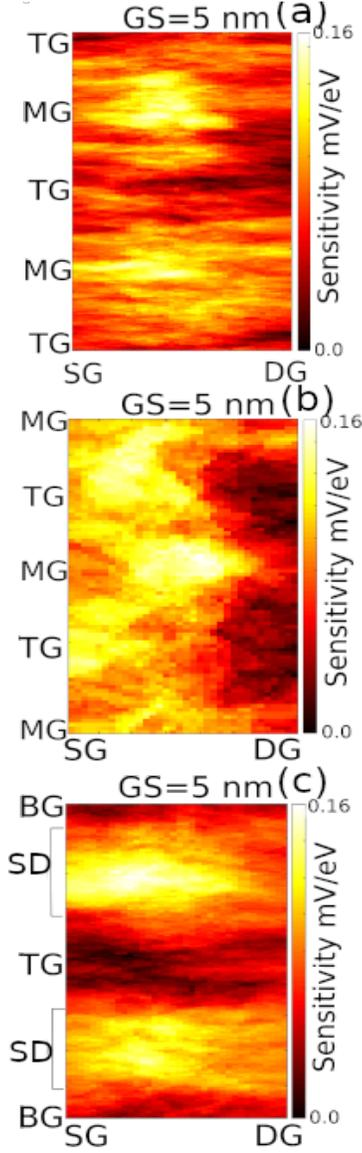
Figure 3. FSM of the  $V_{Th}$  at a GS 5 nm of (a) the 12 nm gate length NSFET, (b) the 10 nm gate length NWFET, and (c) the 10.7 nm gate length FinFET, where SG/DG are the source/drain gate interfaces, TG/MG/BG are top/middle/bottom of the gate and SD are the sidewalls of the gate.
