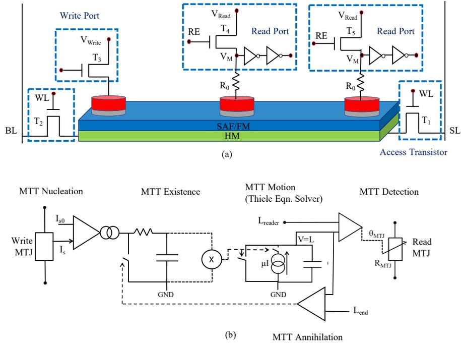
Fig. 2. (a) Generic MTT racetrack memory circuit capable of nucleating, moving, detecting and annihilating skyrmion. (b) Equivalent circuit for MTT nucleation, motion, electrical detection and annihilation.
