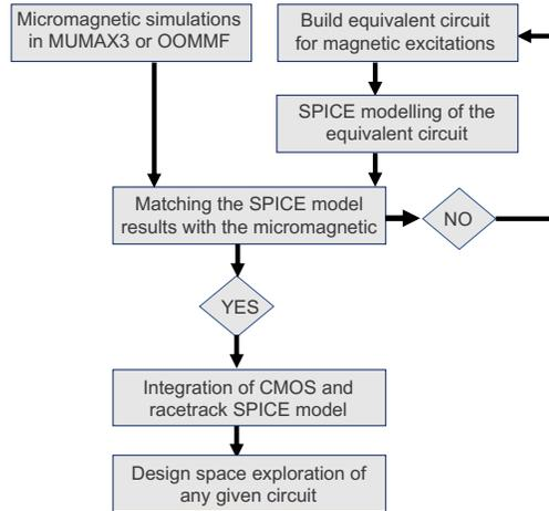
Fig. 1. Micromagnetic to SPICE flow for the compact SPICE model of magnetic topological textures on racetracks.
