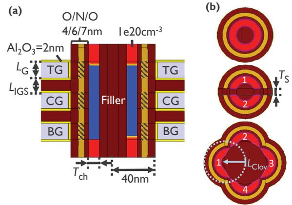
Fig. 1: (a) Simulated three-gate macaroni structure with top, center and bottom word line (TG,CG,BG). The hatched regions indicate where program charge is placed. The pass voltage on TG and BG during read is 7V. (b) Cross-sections, showing single, split and clover channel.
