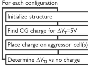
Fig. 2: Simulation flow of 3D TCAD approach to study interference of program charge.
