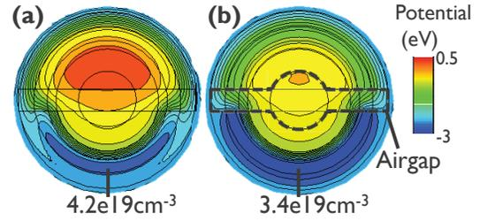
Fig. 7: Electrostatic potential profile of split channel device with program charge on CG2 for  $T_{ch}=10nm$  and  $T_S=5nm$ . (a) No airgap and (b) airgap in the filler region and IGS.
