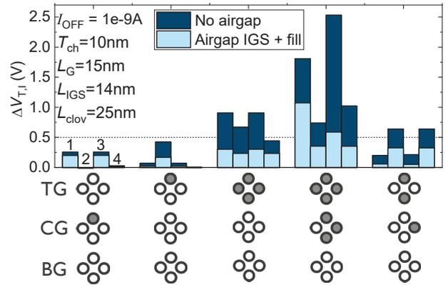
Fig. 9:  $V_T$  shifts due to program charge on various aggressor configurations in a clover channel device and the effect of an airgap in the IGS and filler regions. The impact on  $V_T$  of all channels (labeled “1” through “4”) is shown. For programmed cells, the target  $\Delta V_T$  is subtracted from  $\Delta V_{T,I}$ .
