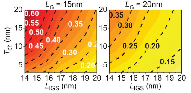
Fig. 4:  $V_T$  shift (V) of CG due to program charge on TG in a single channel device with varying geometrical parameters.
