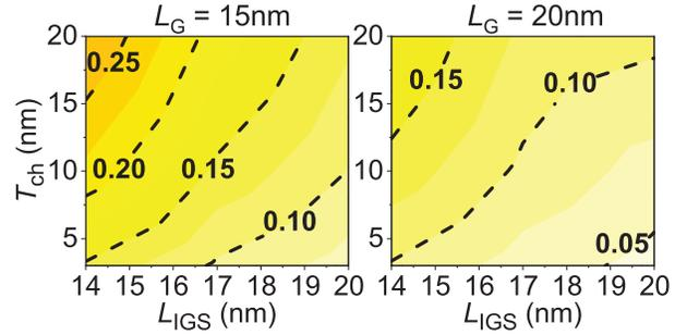
Fig. 5:  $V_T$  shift (V) of CG due to program charge on TG in a single channel device with varying geometrical parameters and an IGS airgap.
