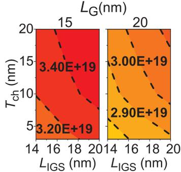
Fig. 3: Required program charge density ( $\text{cm}^{-3}$ ) to obtain a target  $\Delta V_T$  of 5V on CG for varying geometrical parameters.
