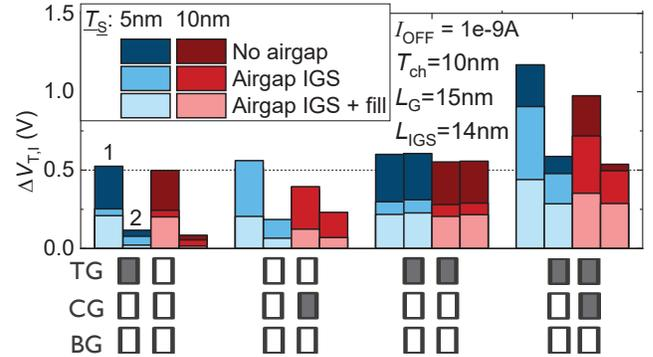
Fig. 8:  $V_T$  shifts due to program charge on various aggressor configurations in a split channel device, for varying channel slit width and the presence of an airgap either in the IGS, or both in the IGS and the filler region. The impact on the  $V_T$  of both channels (labeled “1” and “2”) is shown. For programmed cells, the target  $\Delta V_T$  is subtracted from  $\Delta V_{T,I}$ .
