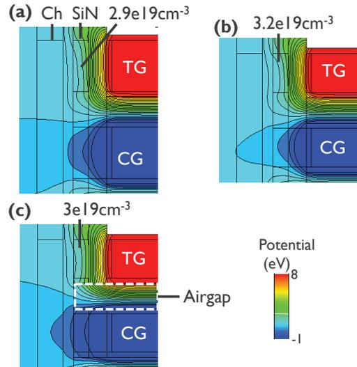
Fig. 6: Electrostatic potential profile in a single channel device with program charge on TG for  $T_{ch}=10\text{nm}$ ,  $L_{IGS}=14\text{nm}$  and (a)  $L_G=20\text{nm}$ , (b)  $L_G=15\text{nm}$  and (c)  $L_G=15\text{nm}$  with an airgap in the IGS as indicated.
