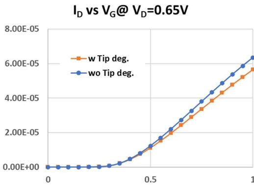
Figure 4. Simulated  $I_d$ - $V_g$  at  $V_d=0.65$  with tip degradation included and with it turned off.
