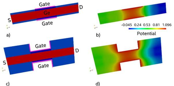
Figure 7. Ge UTB structures and potential profiles for an ideal case (a,b) and more realistic case (c,d) with gate contact on the side of the spacers.
