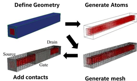
Figure 6. Extending process simulation/structure generation to include generation of both atomic and FEM meshes. Once meshes are generated the contacts and doping are added.
