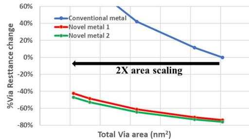
Figure 10. Simulation of via resistances vs via area for novel metal systems compared to conventional metal.
