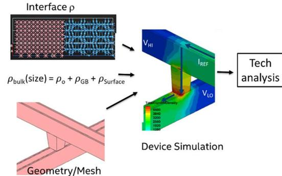
Figure 9. Simulation infrastructure used to estimate Via resistance including interface resistivity, bulk resistivity as a function of size and geometry.
