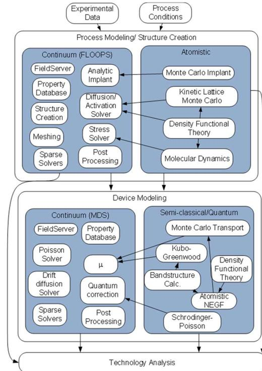
Figure 1. Overview of process and device hierarchy used including typical modeling flows and tool dependencies. Not all dependencies are depicted.
