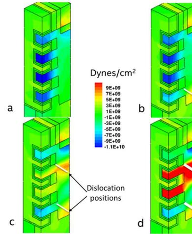
Figure 3. Stress simulation results showing the stress along the current flow direction for a) perfect epi b) one dislocation c) 2 dislocations and d) 2 dislocations with two times the strength (Burgers vector).
