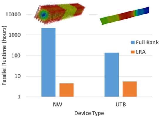
Figure 5. Total parallel CPU time in hours for full rank and LRA simulations of both nanowire (~530x speedup) and ultrathin body (~25x speedup) simulations.
