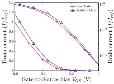
Figure 8.  $I_d$  vs gate bias results for idealized vs realistic structures from Figure 7 relative to current for ideal gate at  $V_{gs} = -0.6$ , which show the impact of more realistic structures on NEGF results.
