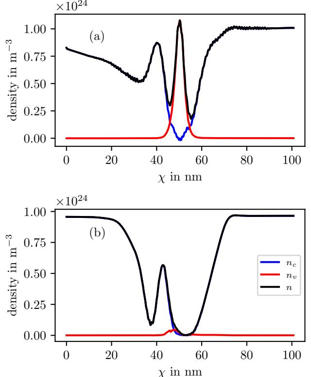
Fig. 3: Carrier density depicted for the peak voltage  $U_{\text{peak}} = 0.13\text{V}$  (a) and  $U_{\text{valley}} = 0.35\text{V}$  (b).
