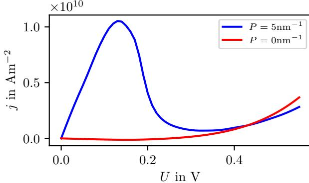
Fig. 2: Current-voltage characteristic for the resonant interband tunneling diode.
