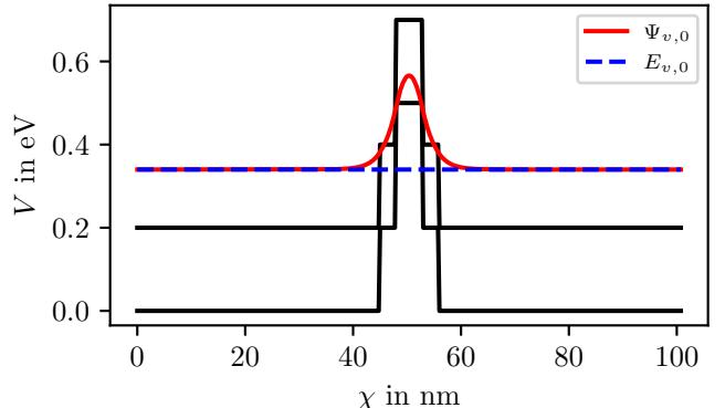
Fig. 1: Band diagram of the resonant interband tunneling diode along with the wavefunction  $\Psi_{v,0}$  (with  $E_{v,0}$ ) of the bounded state within the valence band is depicted.
