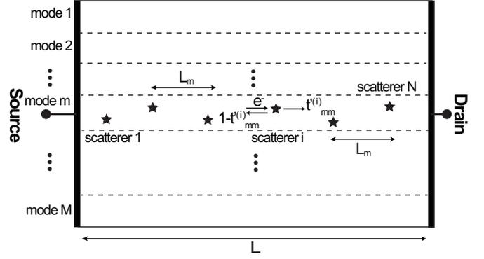
Fig. 2. Schematic elastic scattering model.
