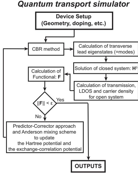
Fig. 1. Flow chart of the self-consistent QT method.  $\epsilon$  is the Poisson residuum tolerance.
