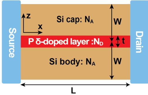
Fig. 3. Schematic model for Si: P  $\delta$ -layer wires.
