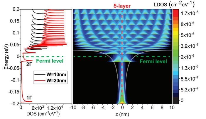
Fig. 4. Left panel: DOS for Si:P  $\delta$ -layer wires with different widths,  $W = 10$  nm and 40 nm. Right panel: LDOS( $z, E$ ) for a 20 nm-width Si:P  $\delta$ -layer wire. For both panels,  $t = 0.2$  nm,  $N_D = 1.2 \times 10^{14}$  cm $^{-2}$  and  $N_A = 1.0 \times 10^{17}$  cm $^{-3}$ .
