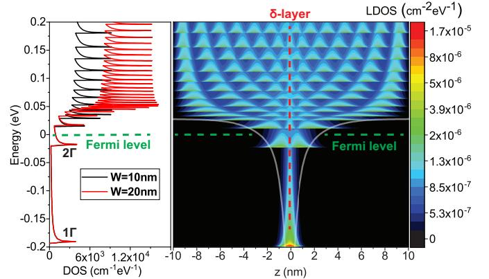
Fig. 4. Left panel: DOS for Si:P  $\delta$ -layer wires with different widths,  $W = 20$  nm and 40 nm. Right panel: LDOS( $z, E$ ) for a 20 nm-width Si:P  $\delta$ -layer wire. For both panels,  $t = 0.2$  nm,  $N_D = 1.2 \times 10^{14} \text{ cm}^{-2}$  and  $N_A = 1.0 \times 10^{17} \text{ cm}^{-3}$ .
