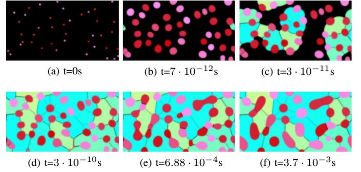
Fig. 2: Temporal evolution of the crystalline state in 2D simulation of the crystallization of an amorphous layer of Ge-rich GST. Amorphous areas are represented in black. The different shades of pink/red stand for crystalline Ge phase and green/blue for GST phase.
