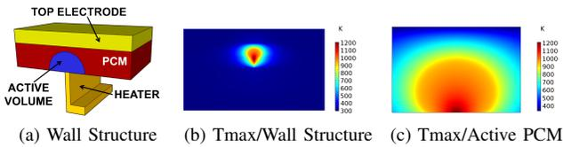
Fig. 3: Joule heating simulation of the Wall Structure
