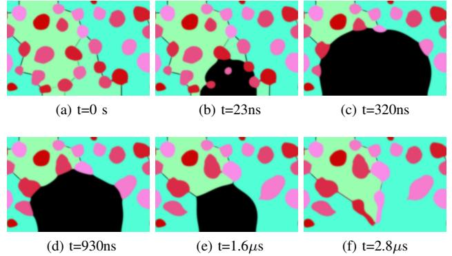
Fig. 4: Temporal evolution of the microstructures during the application of a trapezoidal current pulse to the Wall Structure with the PCM initially in polycrystalline state. The color code is the same as in Fig.2
