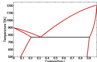
Fig. 1: Phase diagram obtained from the free energy functions
