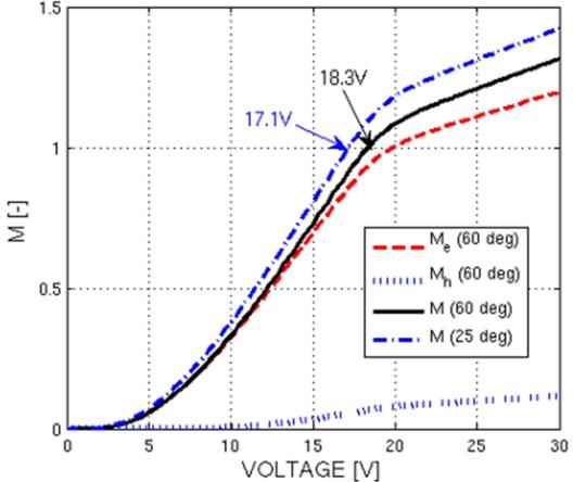
Fig. 3: The mean multiplication factor versus voltage, for two temperatures.  $M=1$  corresponds to  $V_B = 17.1$  volts at 25°C.
