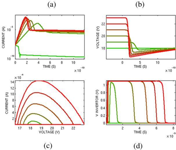
Fig. 4: (a) The current buildup evolution with applied voltage. (b) The voltage drop seen from the SPAD cathode exhibiting a swing. (c) SPAD I-V curve. The breakdown voltage is of 17.1 V (d) The output pulse  $v_{out}$ .
