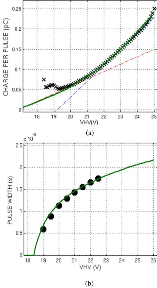
Fig. 7: (a) The charge per pulse  $C_{pp}$  and (b) the pulse width versus VHV; Verilog-A model (solid line) versus measurements (symbols).
