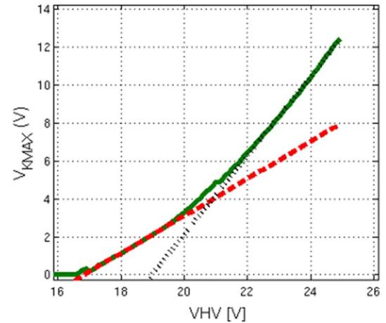
Fig. 6: (a) The swing voltage  $V_{KMAX}$  versus  $VHV$ . Verilog-A model (solid curve),  $V_{KMAX} = VHV - V_B$  (dashed line) and the regime where  $V_{KMAX}$  exceeds the excess bias (dotted line).
