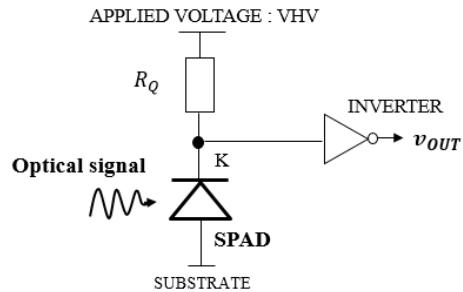
Fig. 1: The cathode terminal of the SPAD diode (sensing node) connected to a quench restor ( $R_Q \sim 500\text{ k}\Omega$ ). During the avalanche, a high generated current gives rise to a detectable swing of the cathode. The inverter allows a square output pulse and reflects the overall time constant of the circuit.
