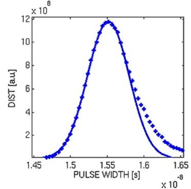
Fig. 5: The pulse width distribution. Solid curve refers to Verilog-A model; symbols to measurements (at VHV= 20.5V and T=60°C).
